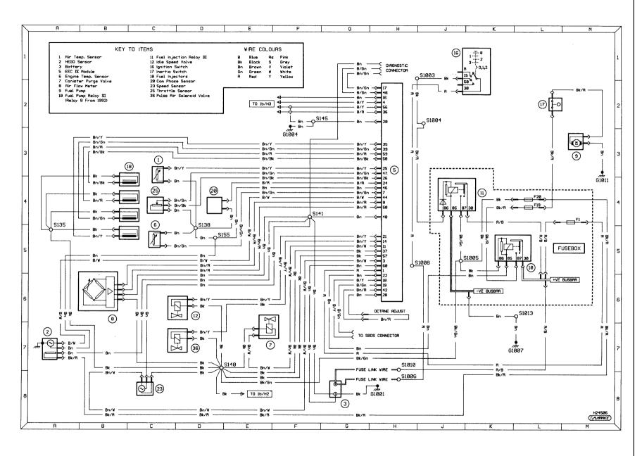
Diagram 1e: DOHC 16-valve fuel injection
